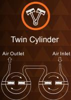
NAVTEK NP4DP 4cfm dual voltage vacuum pump features twin cylinders for high ultimate vacuum down to 15 microns. Integrated cylinder structure coupled with forced oil circulation assure its high performance and reliability. Built-in hook makes it easier to carry to a high workplace.
